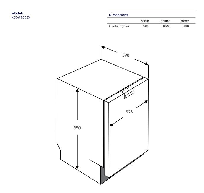
Please note! Dimensions to be used as a guide only. All customers MUST refer to the user manual supplied with the product for detailed installation instructions. © 2021 Electrolux S.E.A PTE. LTD. E\_DIM\_KSE49200SX\_Nov21
