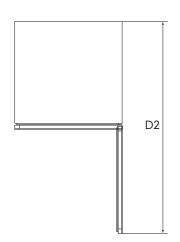
When positioned in a corner area, spacing of at 45+10mm on the hinge side will allow the doors to open enough to enable the removal of bins and shelves.
