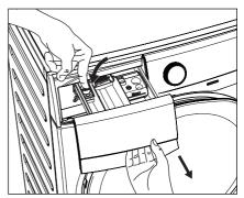
To aid cleaning, the top part of the additive compartment should be removed.
