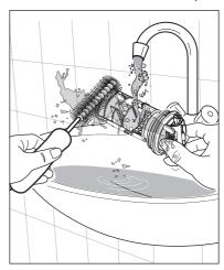
Put the filter back into the housing with exposed section facing up. Make sure that you correctly tighten the filter to prevent leakages.
