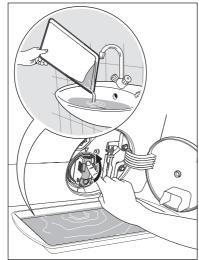
Push back the drainage duct and turn the filter counter-clockwise to remove it.
