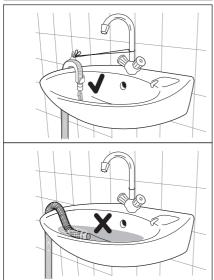
In this case, make sure the end cannot come unhooked when the machine will be emptied. This could be done by tying it to the tap with a piece of string or attaching it to the wall.
