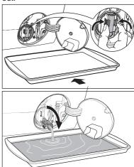
When the container is full of water, put the drainage duct back again and empty the container. Do step 2, 3 again and again until no more water flows out from the drain pump.
