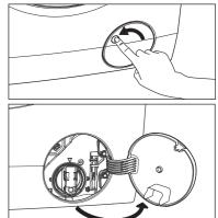
2. Place a suitable water container below the recess of the drain pump to collect the water that flows out.
