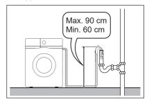
The end of the drain hose must always be ventilated, i.e. the inside diameter of the drain pipe must be larger than the outside diameter of the drain hose.
