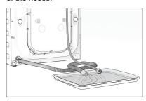
5. When no more water flows, install the inlet hose and the drain hose again.
