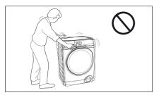
Never place cardboard, wood or similar materials under the machine to compensate for any unevenness in the floor. Install the machine on a flat hard floor. Make sure that air circulation around the machine is not impeded by carpets, rugs etc.
