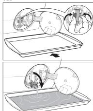
When the container is full of water, put the drainage duct back again and empty the container. Do step 2, 3 again and again until no more water flows out from the drain pump.
