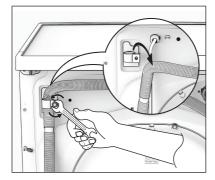
Put the end of the drain and inlet hose in a container. Let the water flow out of the hoses.
